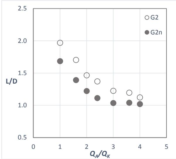
**Figure 6:** Effect of the type of aqueous phase on the slug size.
