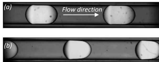
**Figure 2:** Typical slug shapes for: (a) Newtonian fluid G2 (b) non-Newtonian fluid G2n ( $Q_A=120 \mu$ L/min).
