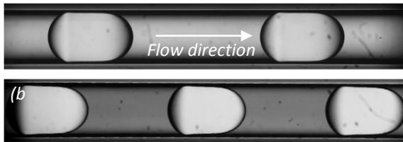
**Figure 9:** Effect of aqueous-phase viscosity on the size, shape and frequency of slugs for (a) *G1n*, (b) *G2n* (non-Newtonian fluids,  $Q_A = 100 \mu\text{L}/\text{min}$ ).
