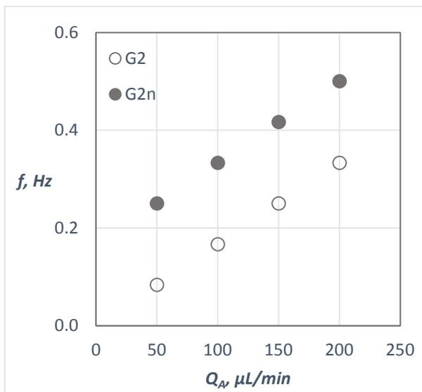
**Figure 11:** Effect of the aqueous-phase viscosity (non-Newtonian and Newtonian) on the slug frequency.
