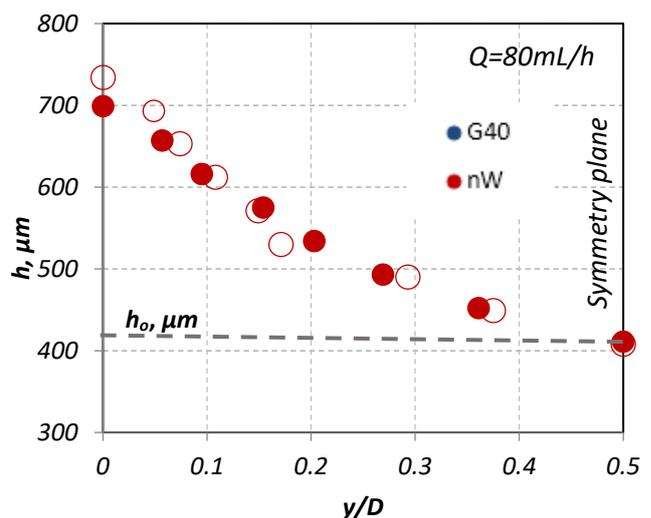
Fig. 2. Comparison of the meniscus between the non-Newtonian (*nW*) and its Newtonian counterpart (*G40*).
