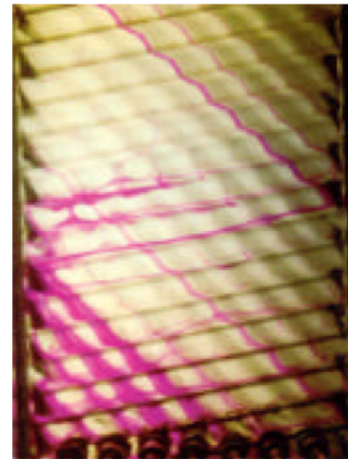
Fig. 3b: Flow visualization by Focke and Knibbe (1986), Re = 125
